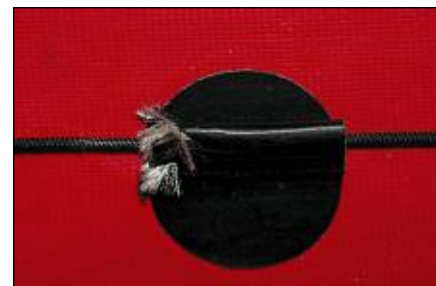
Wear on the spray-deck attachment patches from bashing through ice-pans
