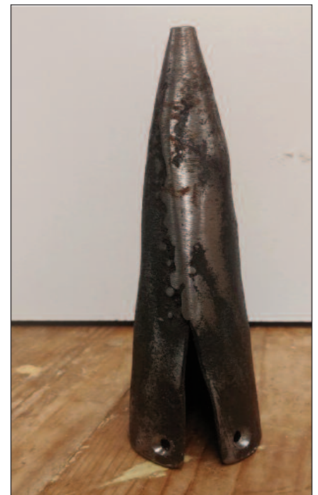
Hand forged, split jacket canoe poling iron.
